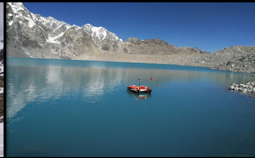
Unmanned boats to measure the volume of water in lakes
